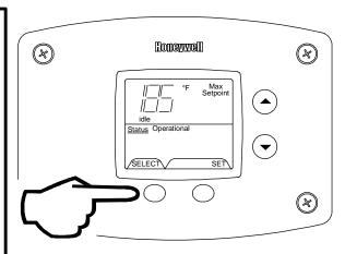
Step 2: Press "Set" button to enter setting mode. "Max Setpoint" will flash to indicate setting mode.
